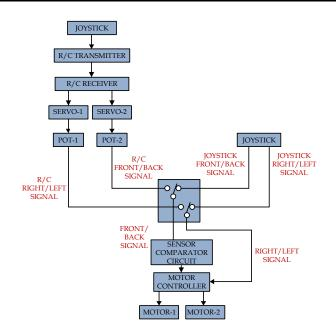
Fig. 17.2. Control diagram.
