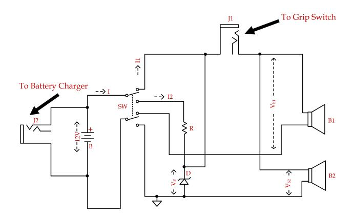
Fig. 17.11. Circuit schematic for sound box.
