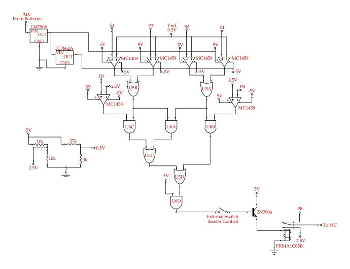
Fig. 17.3. Sensor control circuit.
