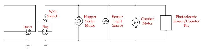
Fig. 17.5. Circuit diagram of electrical components.
