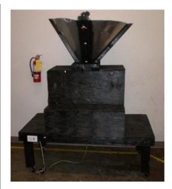
Fig. 17.4. The adaptive can crusher.
